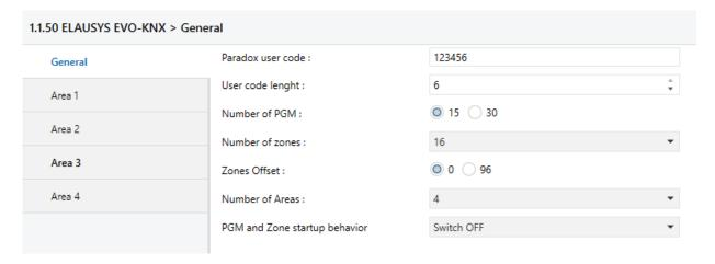
In the general section, enter a valid user code from the Paradox system to enable virtual input and area control.
