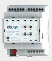
Our KNX Master Switch Actuator is a fully modular actuator system. Extension modules can be plugged in to extend the number channels as needed. Extensions are available for switching, dimming and shutter actuators with various size and power.
